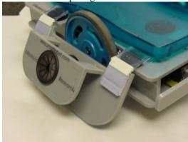
This is how you want the marker to set for the best performance. The pen is inserted from the top with the cap off. It will be stiff the first time.
