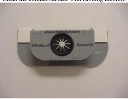
Clean up the two hinges edges. They may be rough from the cutting process. Then, attach the hinges to the holder as shown. Make sure the hinge can bend.
