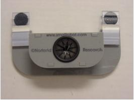
Attach the 4 Velcro pads as shown. Hooks on hinges, loops on robot
